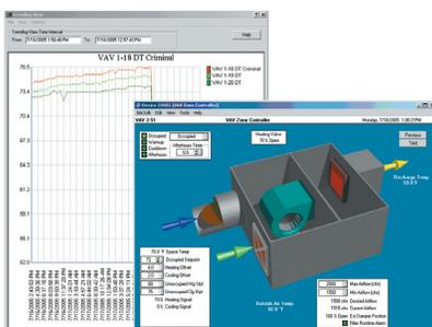
A zone-controlling VAV: Envision for BACtalk's detailed views offer real-time, pinpoint accurate data readings.
